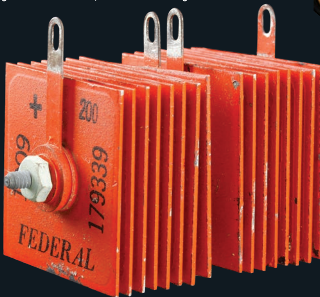
▼ Selenium rectifiers (diodes) predate silicon and germanium varieties, and were much larger.
