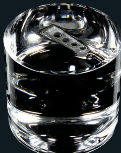
▼ A piece of solid magnesium metal floats on concentrated cesium formate solution, used in oil-well drilling to clear rock chips.
