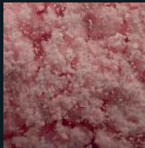
▲ Holmium chloride is the form in which this element is introduced into high-intensity discharge lights, where holmium's spectrum is useful.
