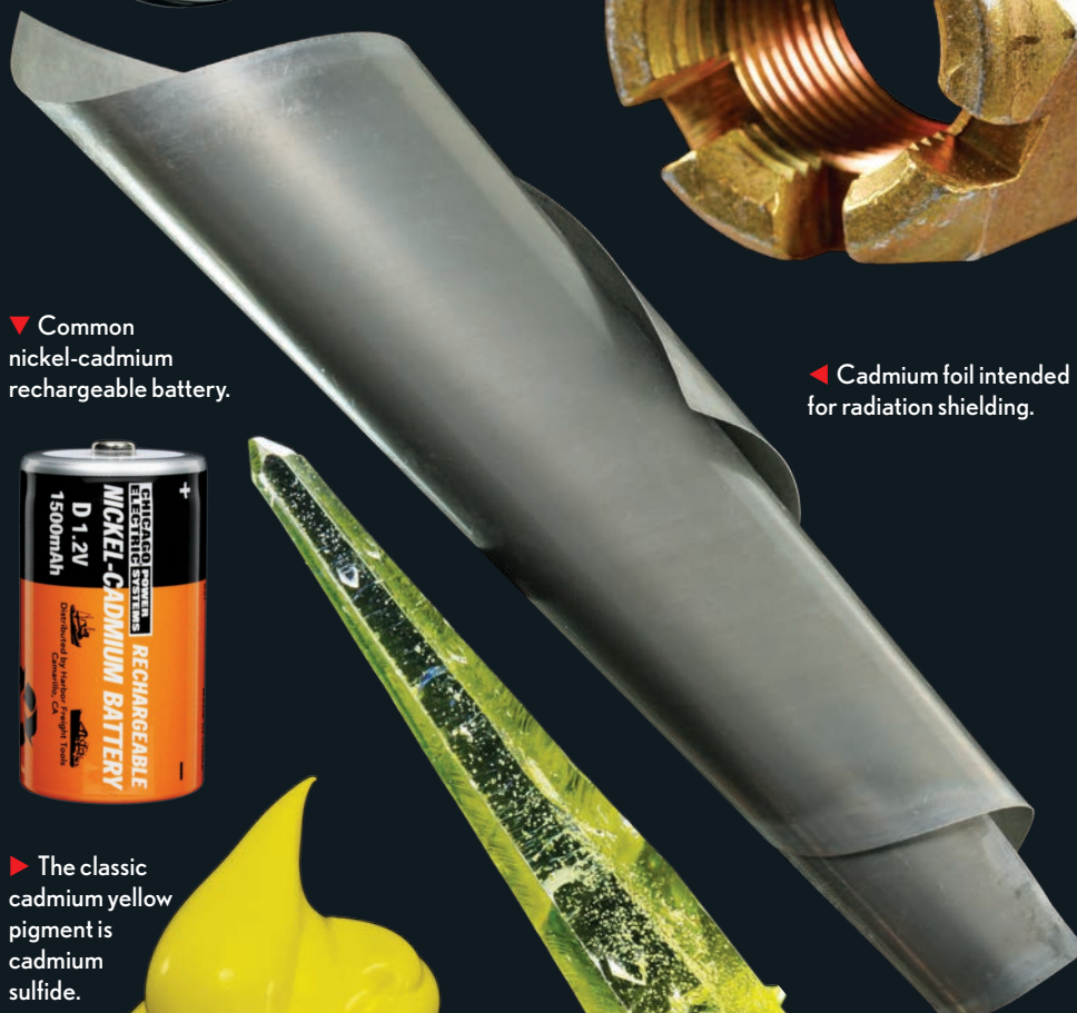
▶ Treatment with dichromate gives these cadmium-plated castle nuts a gold color.
