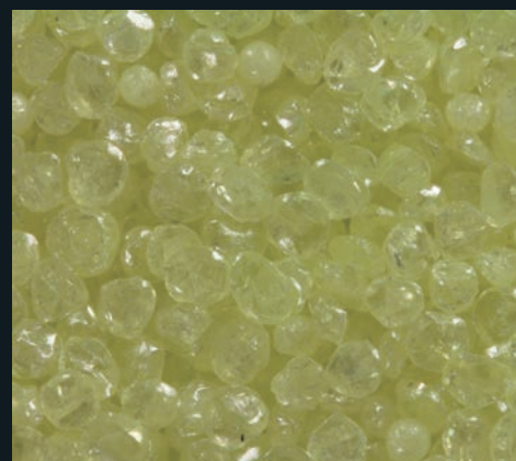
▲ High-purity ytterbium bromide, used in the lighting industry.
