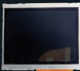
▲ Indium tin oxide conductors are not visible in this LCD screen. That is the point.
