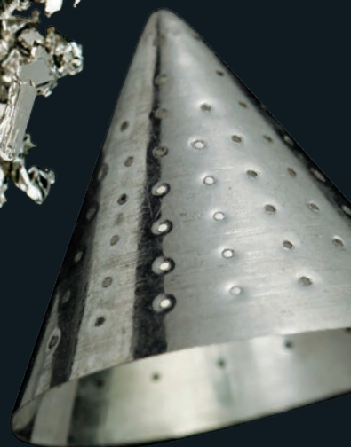
▼ Tiny solid-platinum filter cone, an example of extremely expensive lab ware.
